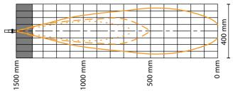
The exact geometry of the sound cone depends on the air-pressure, temperature, humidity and the size of the target.
